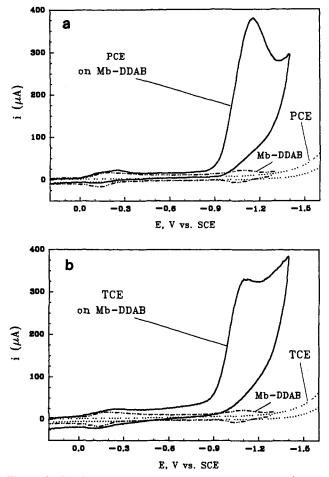
**Figure 4.** Steady state cyclic voltammograms at 100 mV s<sup>-1</sup> in pH 5.5 buffer + 50 mM NaBr: (a) Mb-DDAB films on PG with and without 12 mM PCE, and PCE on a DDAB-PG electrode without Mb; (b) Mb-DDAB films on PG with and without 30 mM TCE, and TCE on a DDAB-PG electrode without Mb.
