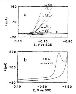
Figure 3. Steady state cyclic voltammograms at 100 mV s<sup>-1</sup> in pH 5.5 buffer + 50 mM NaBr: (a) Mb-DDAB films with trichloroacetic acid at 0, 2.5, 5, 7.5, and 10 mM; (b) reduction peak for 10 mM TCA on a DDAB-PG electrode (no Mb).
