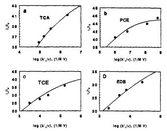
**Figure 8.** Catalytic efficiencies as  $i_c/i_d$  vs log  $(k_1'/\nu)$  for Mb-DDAB films in 10 mM organohalide solutions plotted ( $\bullet$ ) for average  $k_1'$  values (Table 6) for (a) trichloroacetic acid, (b) tetrachloroethylene, (c) trichloroethylene, and (d) ethylene dibromide. Lines represent theoretical predictions simulated in relevant ranges of  $k_1'/\nu$  by using the EC' mechanism with SET approximation (see Experimental Section).
