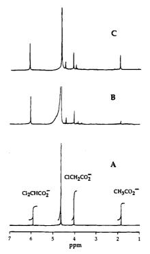
Figure 6. NMR spectra of products from Mb-DDAB-catalyzed reduction of 25 mM TCA in 10 mM deuterated acetate buffer + 50 mM NaBr at pH 5.5 at -0.4 V vs SCE: (a) standards dichloroacetate, monochloroacetate, and acetate, (b) after electrolysis for 5 h, and (c) after electrolysis for 24 h.
