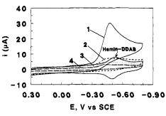
Figure 5. Cyclic voltammograms at 100 mV s<sup>-1</sup> in pH 5.5 buffer + 50 mM NaBr for hemin-DDAB films with and without 10 mM trichloroacetic acid, showing the instability of reduction current after the first scan. (1) first scan, (2) second scan, (3) third scan, (4) fourth scan. CV without trichloroacetic acid present is labeled hemin-DDAB.
