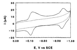
Figure 1. Steady state cyclic voltammograms at 100 mV s<sup>-1</sup> in pH 5.5 buffer + 50 mM NaBr: dashed line, bare PG electrode with 0.5 mM Mb in solution; solid line, fully loaded Mb-DDAB film in buffer containing no Mb.
